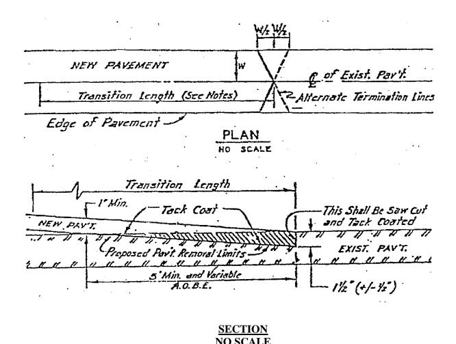
NOTES: The length of transition will be determined by existing gradients, depth of new asphalt courses and A.O.B.E. Areas that are over excavated or rough cut shall be brought up to "Proposed Pavement Removal Limits" with an acceptable leveling course. Tack coats shall meet the requirements of Subsection 702-340l.
