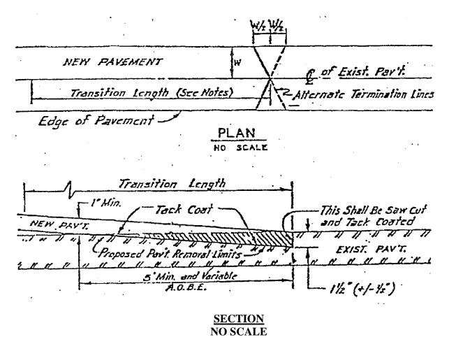
NOTES: The length of transition will be determined by existing gradients, depth of new asphalt courses and A.O.B.E. Areas that are over excavated or rough cut shall be brought up to "Proposed Pavement Removal Limits" with an acceptable leveling course. Tack coats shall meet the requirements of Subsection 702.
