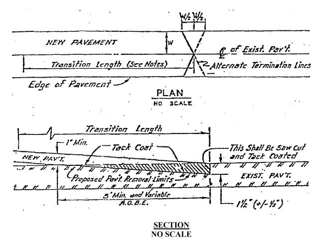
NOTES: The length of transition will be determined by existing gradients, depth of new asphalt courses and A.O.B.E. Areas that are over excavated or rough cut shall be brought up to "Proposed Pavement Removal Limits" with an acceptable leveling course. Tack coats shall meet the requirements of Subsection 702-3401.
