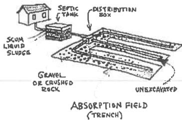
A properly designed, installed and maintained septic system is an efficient method of wastewater treatment, adequately treating sewage before it mixes with ground waters.
