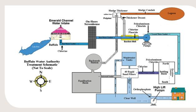
**Sedimentation**: The process of suspended solid particles settling out (going to the bottom of the vessel) in water.
