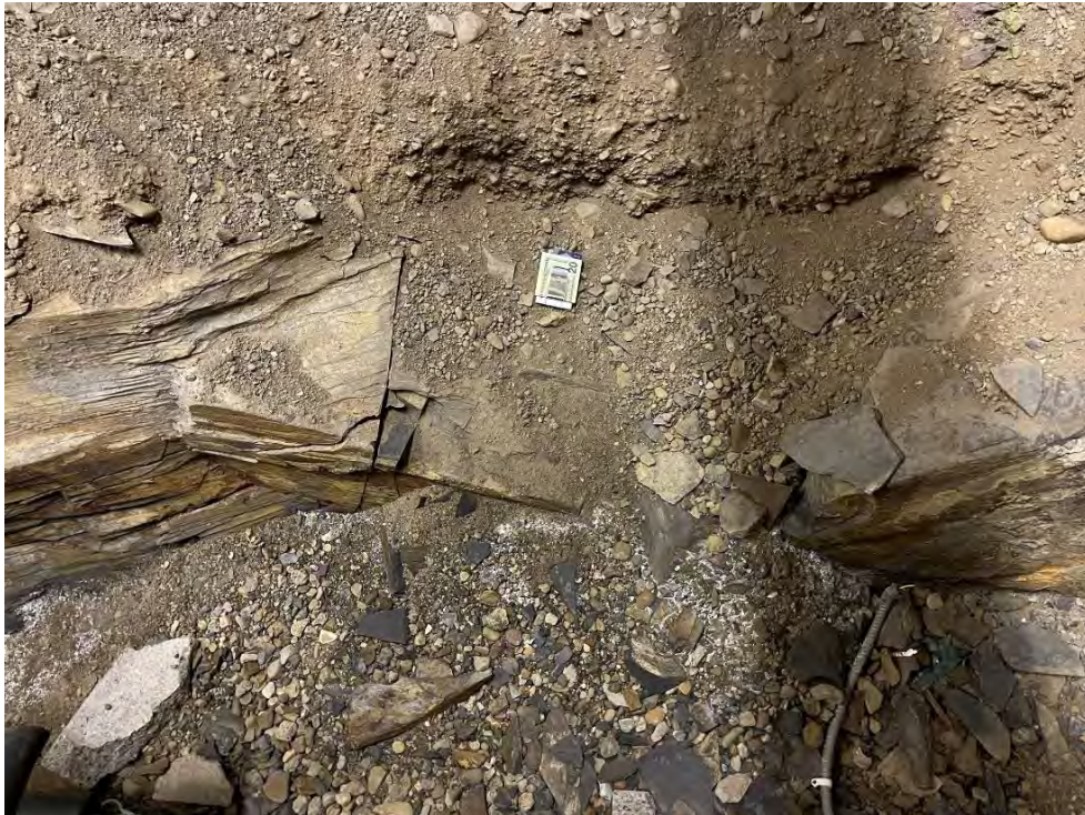
Thin-bedded and jointed shale exposed in a mechanical room at the existing stadium, approximately 1,000 feet east of the proposed stadium. Similar rock mass conditions are expected at the proposed stadium location.
