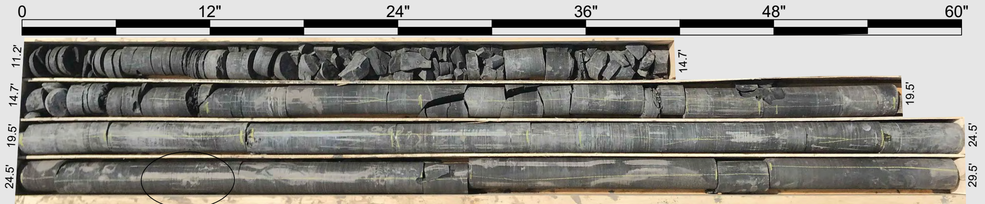
Sample 22-294 Unconfined Compressive Strength: 2351.3 PSI
