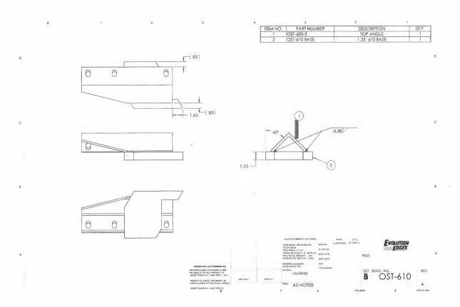
Steel moldboard shoes 8" or 12" center to fit 6" top punch, part # OST-610-60 or equal: See drawing below
