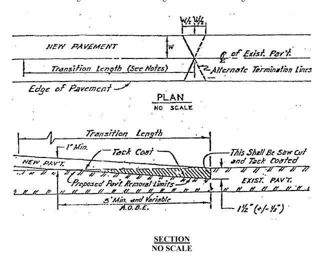
NOTES: The length of transition will be determined by existing gradients, depth of new asphalt courses and A.O.B.E. Areas that are over excavated or rough cut shall be brought up to "Proposed Pavement Removal Limits" with an acceptable leveling course. Tack coats shall meet the requirements of Subsection 702-340l.
