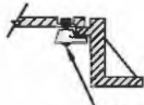
B-B ROTATE CAM TO LOCK COVER (DR EQUAL) LOCKING DEVICE IF REQUIRED
