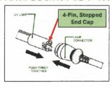
UV bulb type: 4-Pin, Single Ended, High Output, T5 Quartz Glass, Keyed Ceramic
